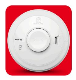
Ei3014 Heat Alarm was installed across the properties to provide enhanced detection for heat build-up from large flaming fires. The alarm is equipped with a tried and tested high-performance thermistor heat sensor to provide a fast response when the trigger temperature of 58°C is reached. Additionally, it can differentiate smoke from steam to help reduce the number of false alarms activated.
